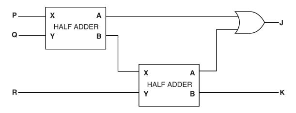
Complete the following truth table for this logic circuit.
